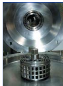
Classifier wheel arrangement for small scale production plant.
