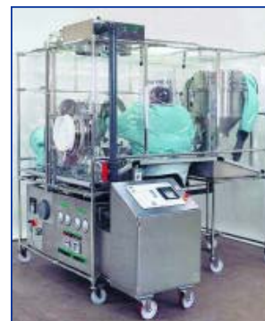
Atritor M8 micronising mill for low OEL steroids inside an ACE (Applied Containment Engineering) isolator.
